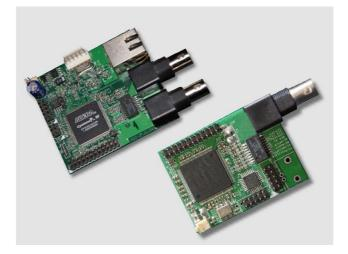
ASI output board provides TV Operators with "budget" solution of getting ASI (Asynchronous Serial Interface) stream for TV broadcasting.
